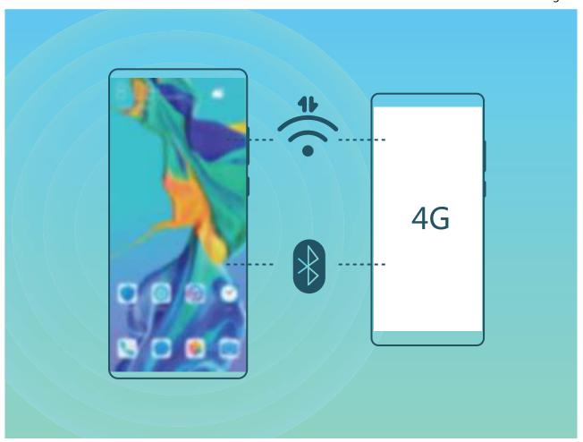
Use personal hotspot to share mobile data: Open Settings and go to Wireless & networks > Personal hotspot. Set Device name and Password, then enable the hotspot to use it.
