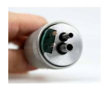
Clean the measuring probe with compressed air and grease the sealing rings with vaseline.
