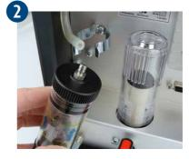
Disconnect the water trap from the hoses and disassemble it.
