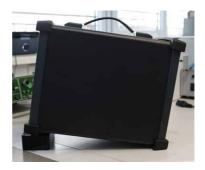
Open the drain cock and tilt the instrument for a few minutes to allow any condensate to flow out.
