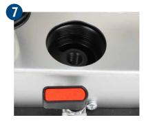
Clean the filter pot with a soft cloth (remove sealing ring before). Insert the sealing ring into the filter pot and screw in the tie rod with filter unit until the filter element is firmly seated, resp. can no longer be turned. Then screw the plastic container on by hand.
