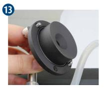
Check sealing ring for cleanliness and, if necessary, grease with commercially available vaseline.
