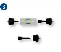
Unscrew the cylinder from the upper part and check the holes as well as the inlet/outlet for permeability. If necessary clean the parts with compressed air.
