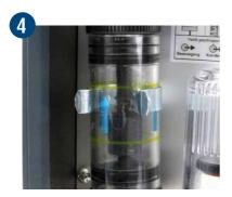
Assemble the water trap and insert into the holder with the arrow pointing upwards.
