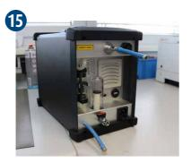
Attach the enclosed hoses to the dust measuring instrument and probe as shown.
