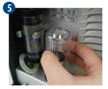
Unscrew the plastic container of the filter unit by hand. Pay attention to the sealing ring!
