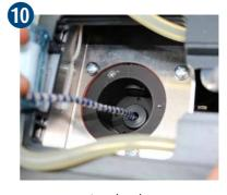
Open measuring chamber cover. Clean the dust channel with the pipe cleaner.
