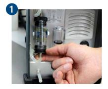
Loosen the water trap from the holder.
