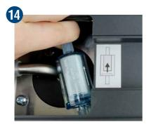
Replace the pump filter if needed. Replace in the direction of the arrow.
