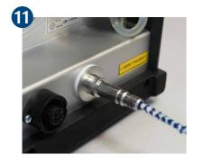
Clean the connection for the heated line with the pipe cleaner up to the measuring chamber.
