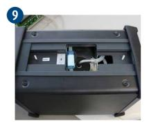
Turn instrument upside down and loosen bottom cover.
