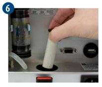
Unscrew the tie rod with filter element and replace the filter if necessary.
