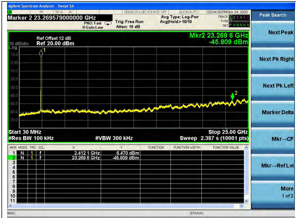
(30MHz to 25GHz, Channel 1, 802.11b)
