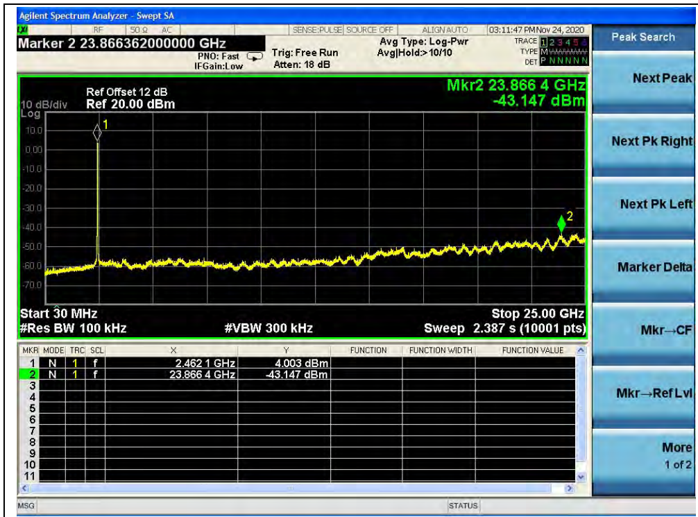
(30MHz to 25GHz, Channel 11, 802.11g)
