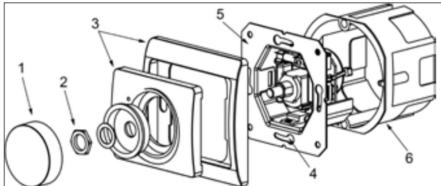
1. Remove the speed regulator's control knob (1).
