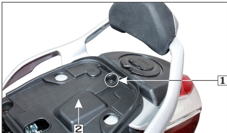
(1) Bolt (2) Fuel tray sub assembly
