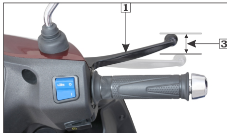
(1) Front brake lever (3) Free play: 10-20 mm
