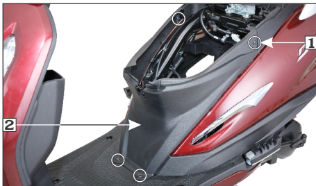
(1) Center cover screws (2) Center cover
