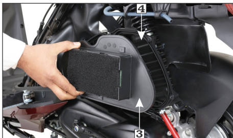
(3) Air cleaner element holder component
