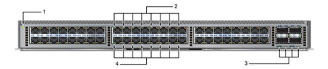
1 Status LED 3 10G/40G Port LEDs 2 10G upper port LEDs 4 10G lower port LEDs
