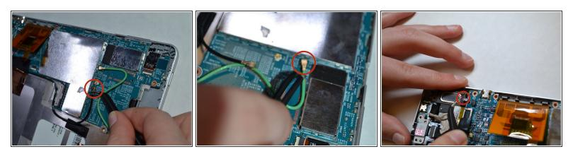
• Disconnect all cords, wires, and resistors from the motherboard using tweezers.
