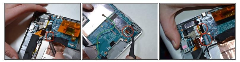
Continue to disconnect all resistors attached from the motherboard, using tweezers.
