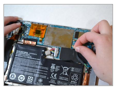
• Remove the black tape connecting the battery to the motherboard.
