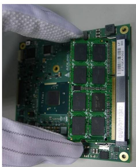
Step 2: Remove the protective membranes from the thermal pads.
