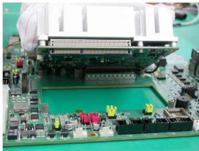
Then press down on the module until it is firmly seated on the carrier board.
