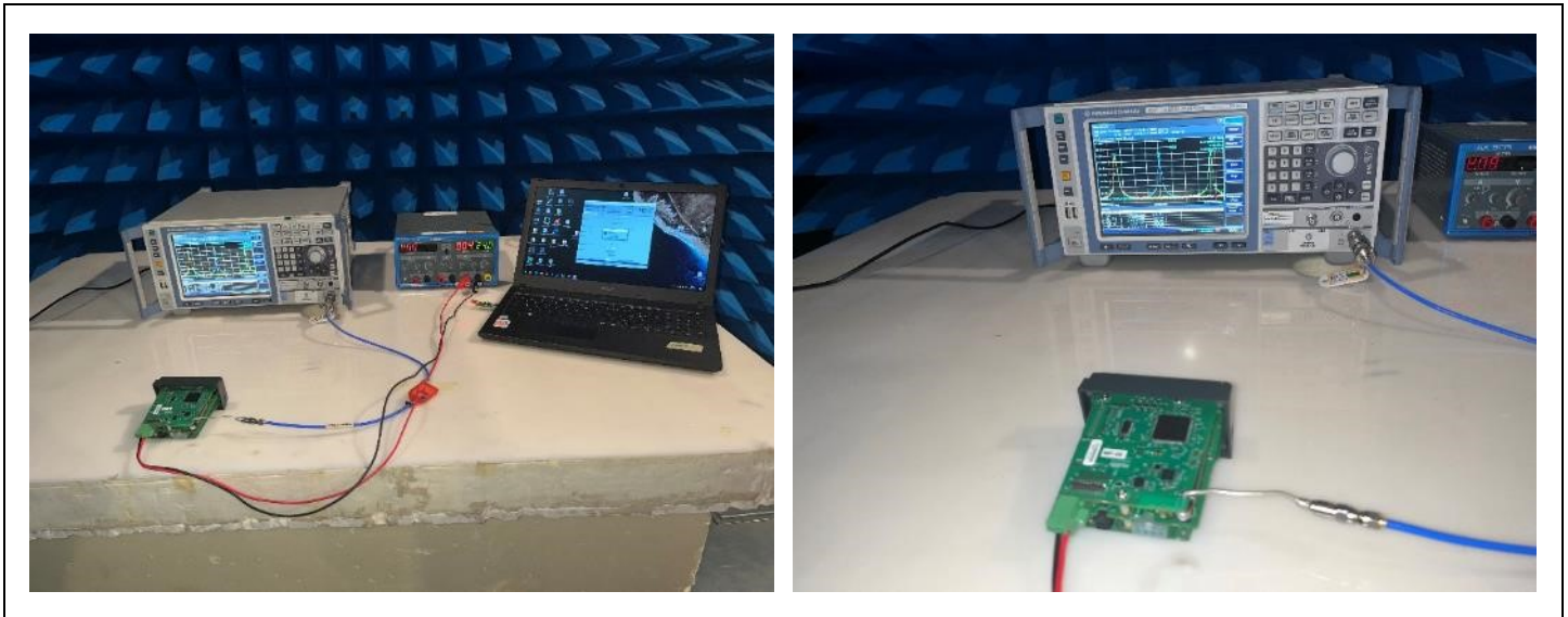
Photograph for Unwanted Emission into non-restricted frequency bands at the band edge
