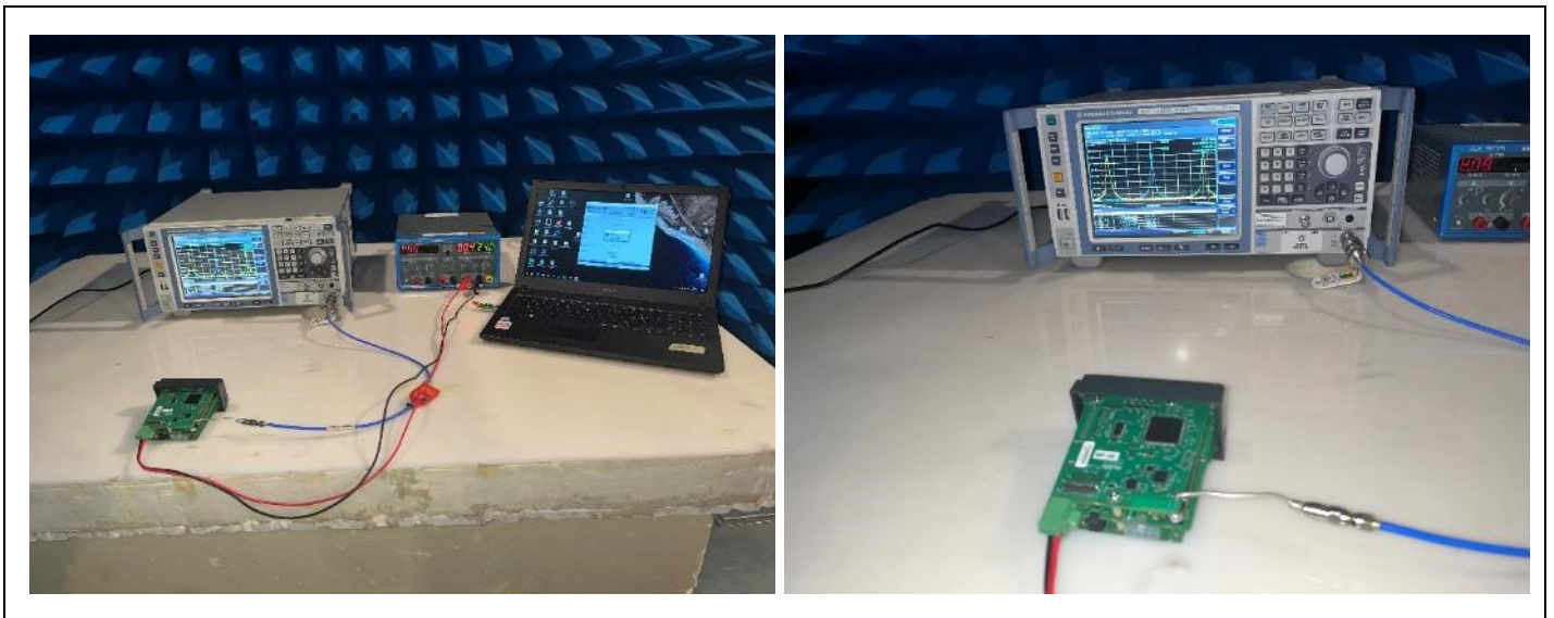
Photograph for Maximum Conducted Output Power
