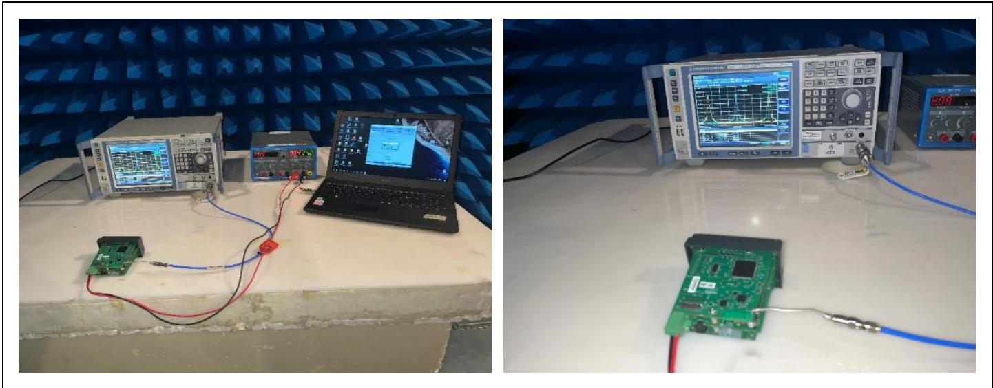
Photograph for Power Spectral Density
